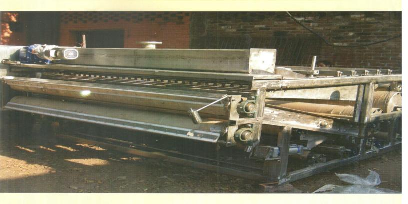
Belt Filter Press is a Continuous sludge dewatering device which uses chemical conditioning, gravity drainage and mechanically applied pressure to dewater sludge.
